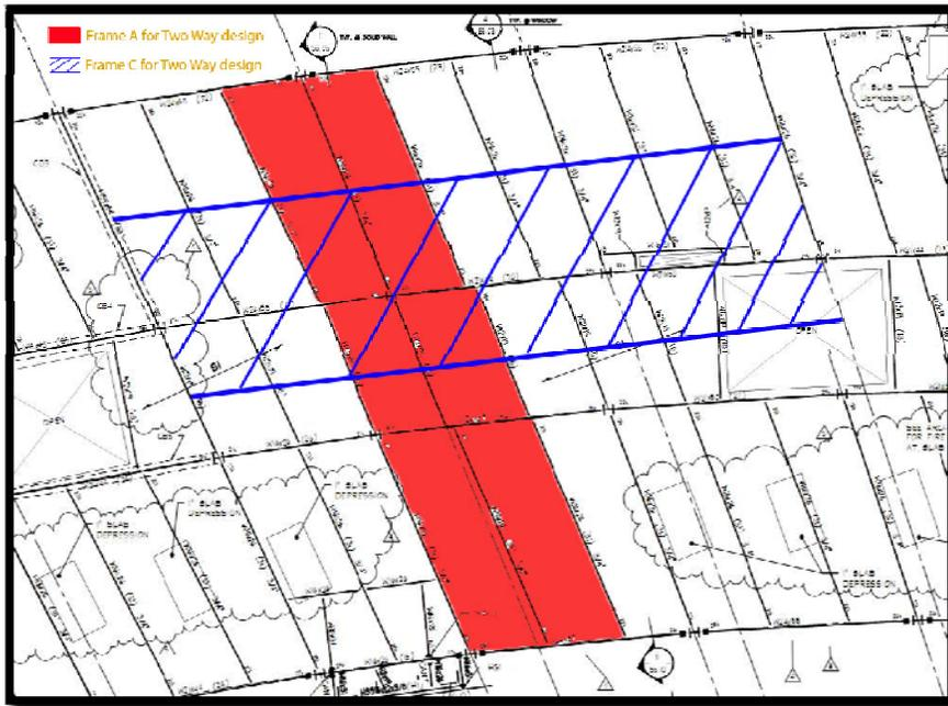
Figure 3: Designated frames for two-way flat slab design
