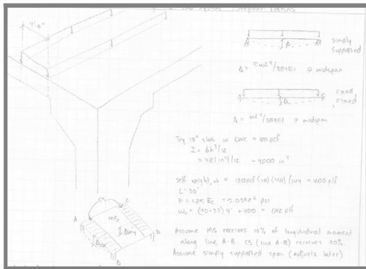
Figure 12: Graphic for deflection of two way flat slab
