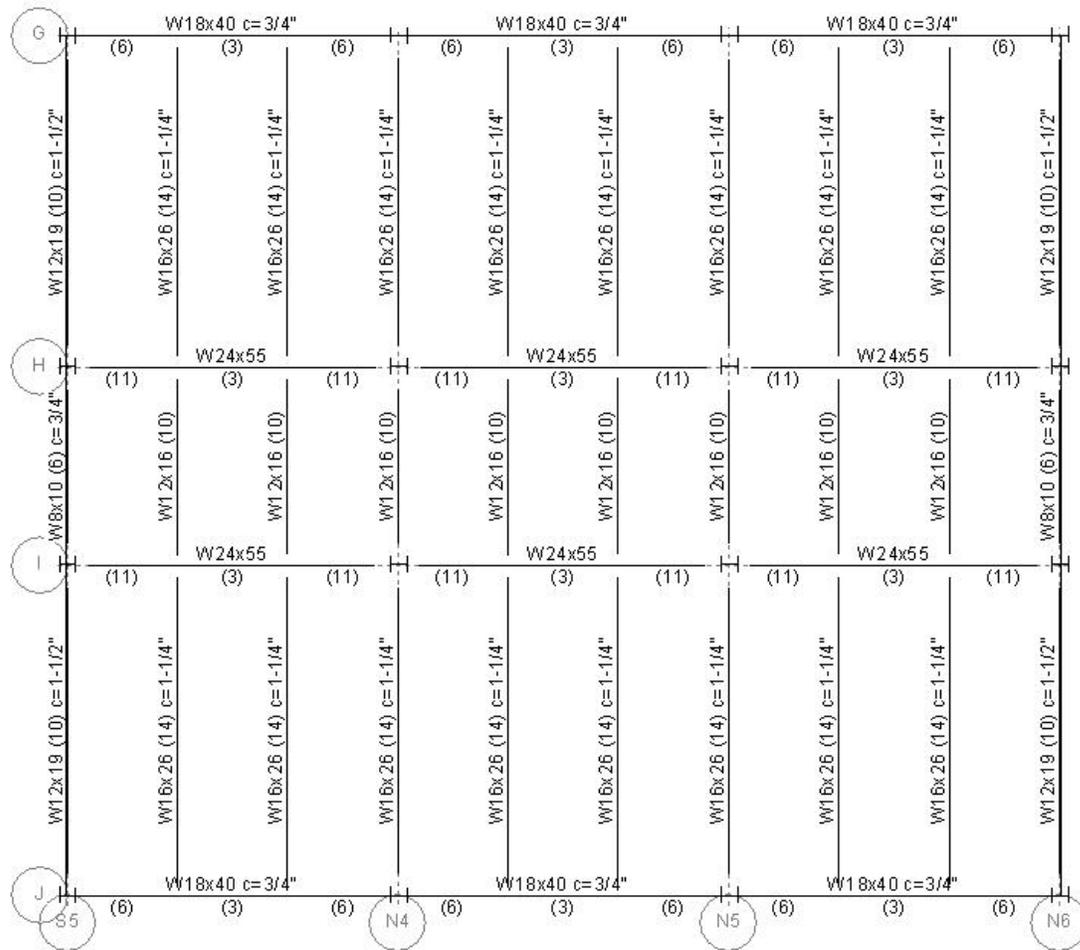
Figure 9: Composite beam and composite girder designs from RAM Structural System
