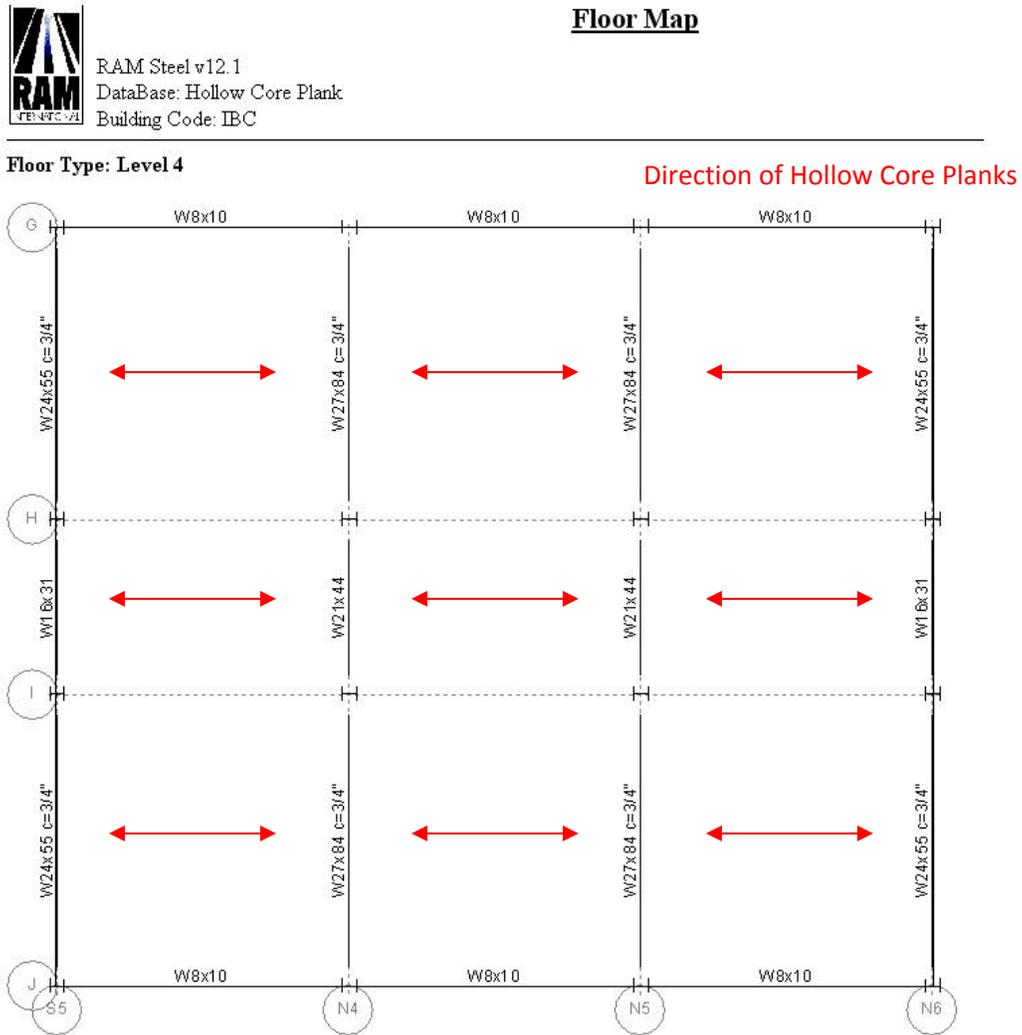
Figure II: Design of steel girders for hollow core plank system
