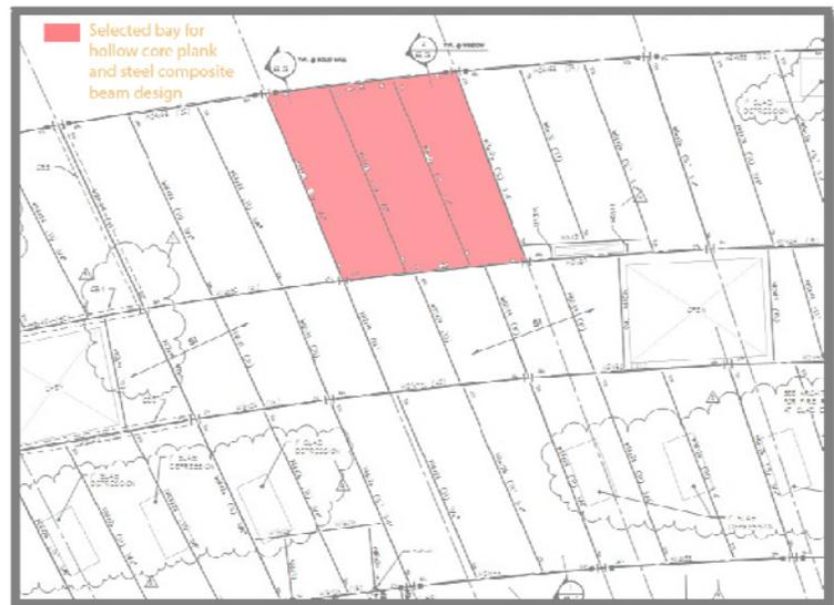
Figure 4: 30'x30' bay used for final comparison of all floor systems
