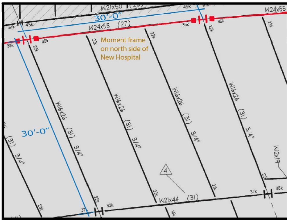
Figure 8: Current framing plan for composite beam floor system
